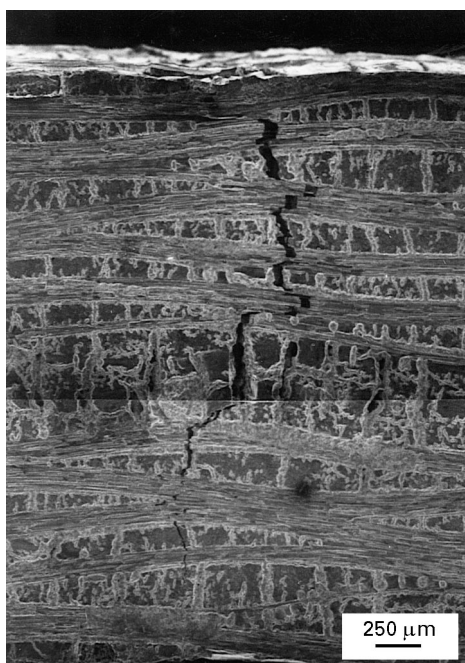
Figure 8 Scanning electron micrograph, showing crack propagation in an untreated specimen; four-point bending.
